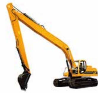
Long Boom Excavator
